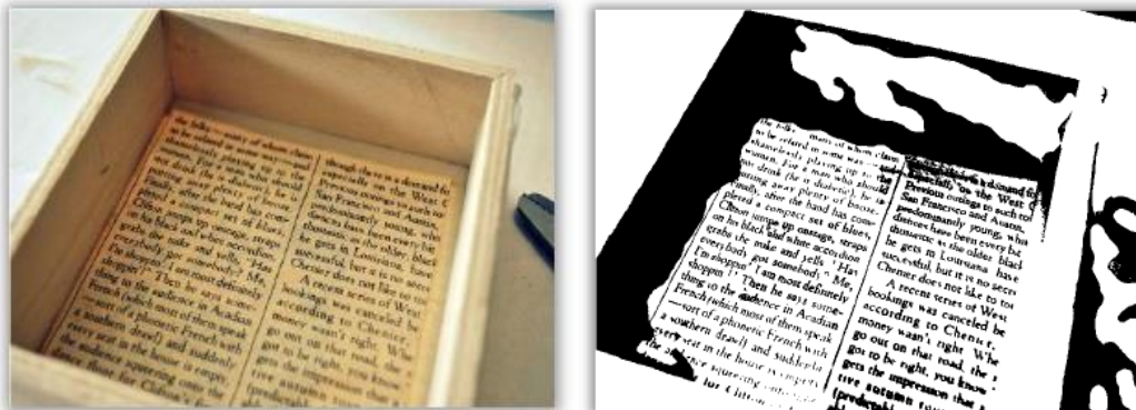
Figure 2. Example of text separation using voting-based image binarization: original image (left), binarized image (right). Image taken from [7]
