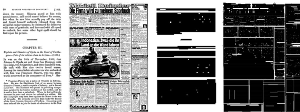
Figure 4. The result of document layout analyze: simple and complex document original images (left), voting-based layout analyze results (right). Image taken from [16]
